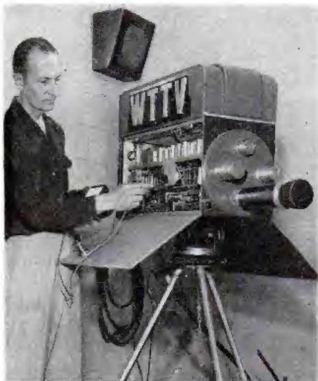
Above, vital to a small station is a machine to show movies, opaque slides, transparencies and title "roll downs" through one iconoscope. Below, the original homemade pickup camera at WTTV
